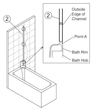
Install the wall channel so it is vertical, and the outside edge is vertically in line with 'Point A' (see drawing).
