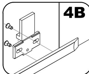
Install the door onto the bottom hinge.
