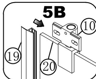
Install the vertical door seals along the whole height of the door, and fit the bottom drip strips in between.
