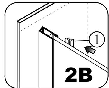
Start at the bottom and work up with the supplied roller tool.
