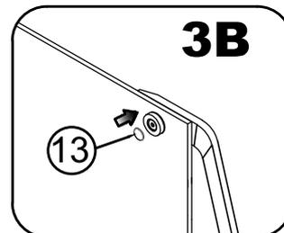
Fit cap to the wall channels.
