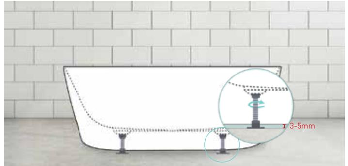
3. Carefully tilt the bath on its side & connect it to the drain outlet. We recommend using a *Decina Flexible Connector*. Ensure the Flexible Connector is cut to the correct length for easier installation & to prevent drainage issues.
