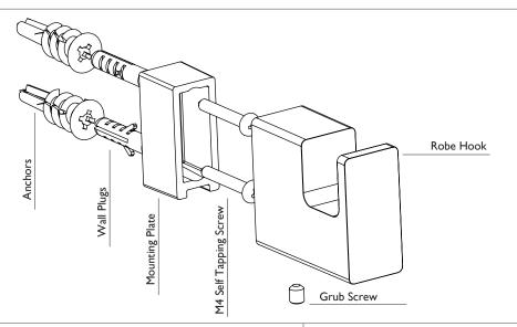
Place fixing plate where Robe Hook is to be mounted. Mark center position of slotted holes.
