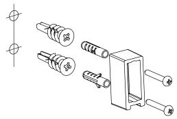
Place mounting plate in position. Insert screws and tighten firmly with a Phillips Head screwdriver 3 Ensure Mounting Plate is level.
