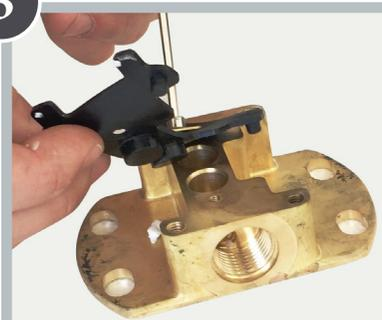
When ready to fit mixer to base, remove rubber seal from top of base plate
