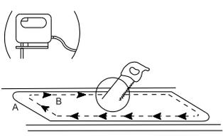
CUT THE SINK CUT OUT TO THE INSIDE OF THE CUT OUT TEMPLATE
