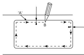
USING THE CUT OUT TEMPLATE PROVIDED, MARK THE CUT OUT LINE ON THE BENCHTOP
