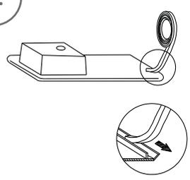
FIT GASKET TO SINK ENSURING DOUBLE THICKNESS AT THE CORNERS USING THE SEALING TAPE SUPPLIED.
